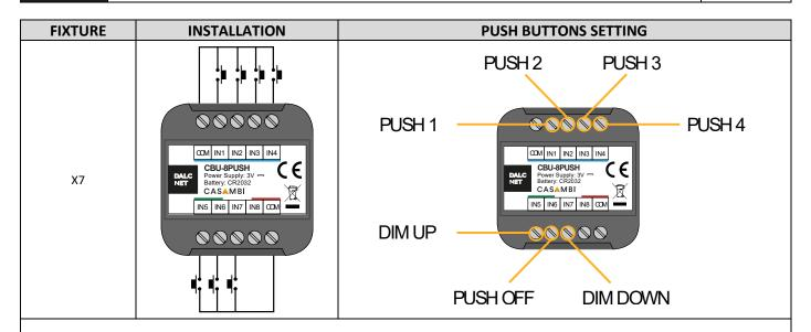
With this fixture it is possible to set up maximum 4 N.O. push buttons. Each push button can control a luminaire, control a group of luminaires, control a scene or an animation. This configuration is possible to set by Casambi APP. By means of two push buttons configurated for dimming it is possible to dimming UP or dimming Down the selected luminaire.
