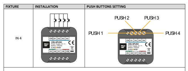
With this fixture it is possible to configure up to 4 N.O. push buttons. Each push button can control a luminaire, control a group of luminaires, control a scene or an animation. This configuration is possible to set by Casambi APP.
