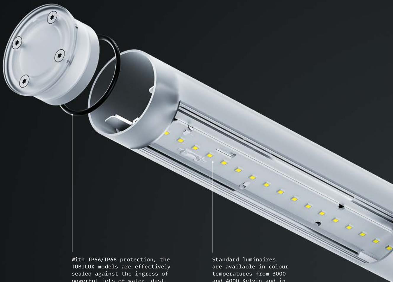
With IP66/IP68 protection, the TUBILUX models are effectively sealed against the ingress of powerful jets of water, dust and other foreign bodies. The maximum available protection against the ingress of water is offered by TUBILUX and TUBILUX XT with IPX9K degree of protection. With IK10, these exceptionally durable luminaires easily withstand impact energy of up to 20 joules.
