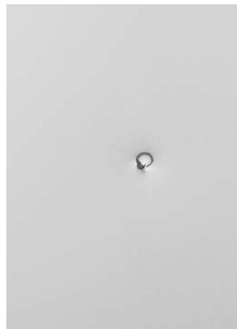
Surface illuminated with diffuse light – faults are barely visible
