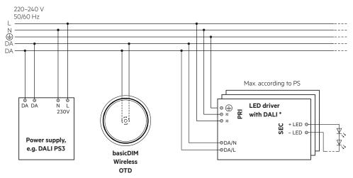
$<sup>^{\</sup>ast}$  Max. 4 single / group addresses (A0 ... A3 / G0 ... G3) controllable, depending on the device profile of the basicDIM Wireless module.
