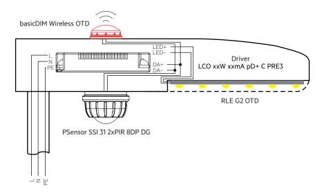
The basicDIM Wireless OTD supports the Zhaga connectivity standard for Plug&Play luminaire extensions. This allows a toolless and flexible integration in luminaires.
